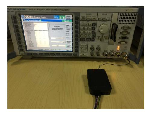
Spurious Emission Test Setup (Below 1GHz)
